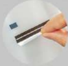
Heat-sealing the band on each end
